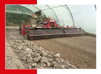
Built with a working width from 360 to 500 cm, required power from 140 to 240 HP and working depth from 15 to 30 cm.
